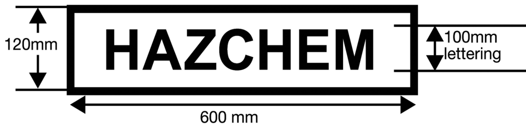
Figure 13.1 Form and dimensions of outer warning placard
