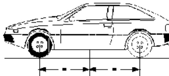
Ground clearance at the mid-point between 2 axles
