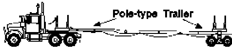
Typical pole-type trailer
