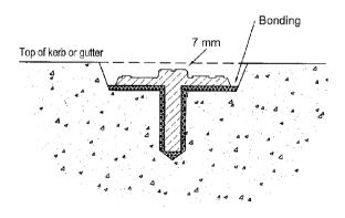
Fixation is by drilling and bonding with a sutable epoxy- resin compound
