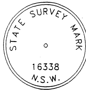
PERMANENT MARK TYPE 3 (State Survey Mark)
