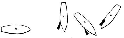
If A sees a mast-head light above the green light A knows that the vessel is a steam vessel and is either approaching her in the same direction as B or is crossing to starboard in some direction as D D D.
